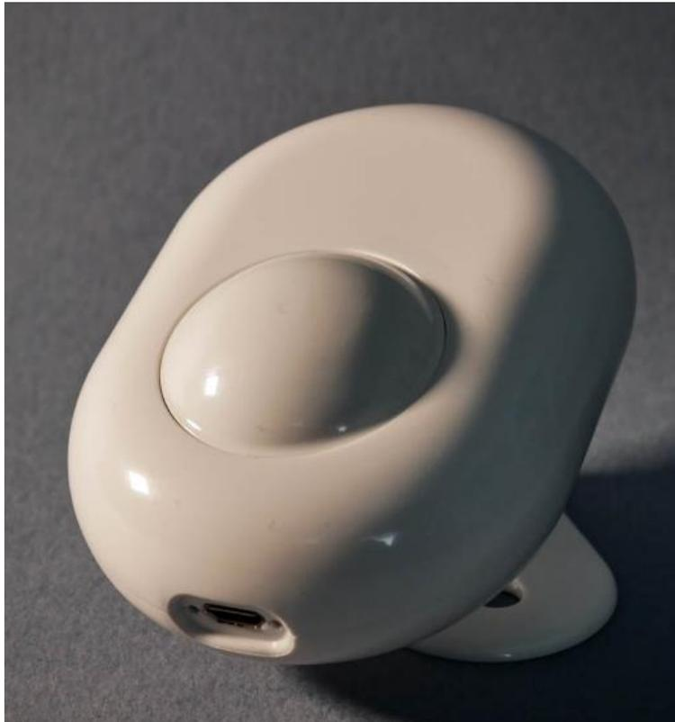
Shelly Motion Sensor does provide a “free” vibration and lux sensor. The vibration sensor will report when the device is moved. This is good for security devices where the concern is that the intruder is trying to defeat the systems that are detection his/her presence. It may be more important with the large Shelly Motion, but in general I doubt if intruders are looking for sensors in one house.
