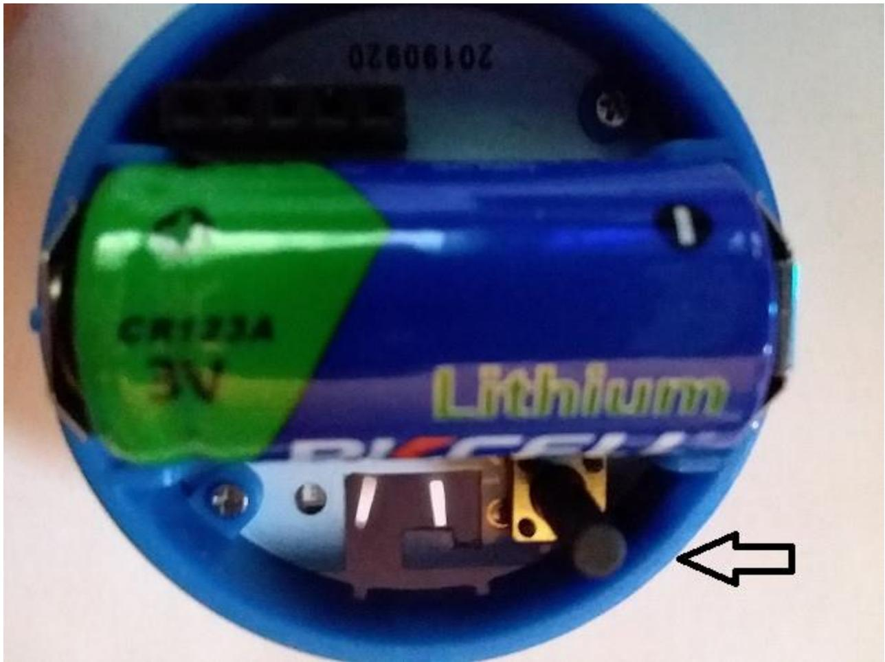
Figure 16 Shelly H&T Battery and Button Locations
