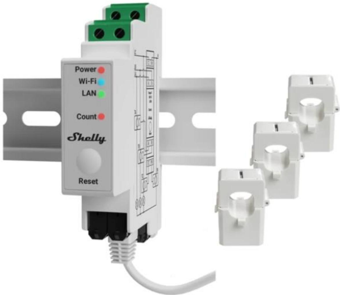
The Shelly Pro 3EM is a status-only device that measures energy in each of three phases and provides a temperature measurement. The temperature will be selected to be the one that is F vs. C based upon HS settings. The HS Device and Features are shown in Figure 49.
